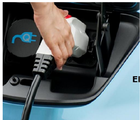
The J1772 connector will be the standard charging plug for all new electric vehicles. Photo courtesy of Nissan.
