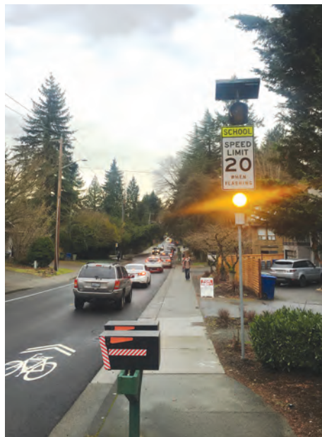
The levy funded the first school zone flashing beacon around a high school, this one located on 108th Avenue Southeast near Bellevue High School.
