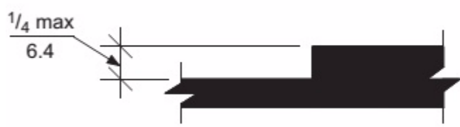
FIG. 303.2 VERTICAL CHANGES IN LEVEL
